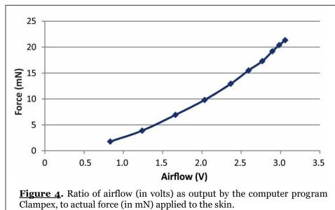
force plate to calibrate the actual amount of force delivered, in mN, compared to the computer readout, in volts (V), (Figure 4).
