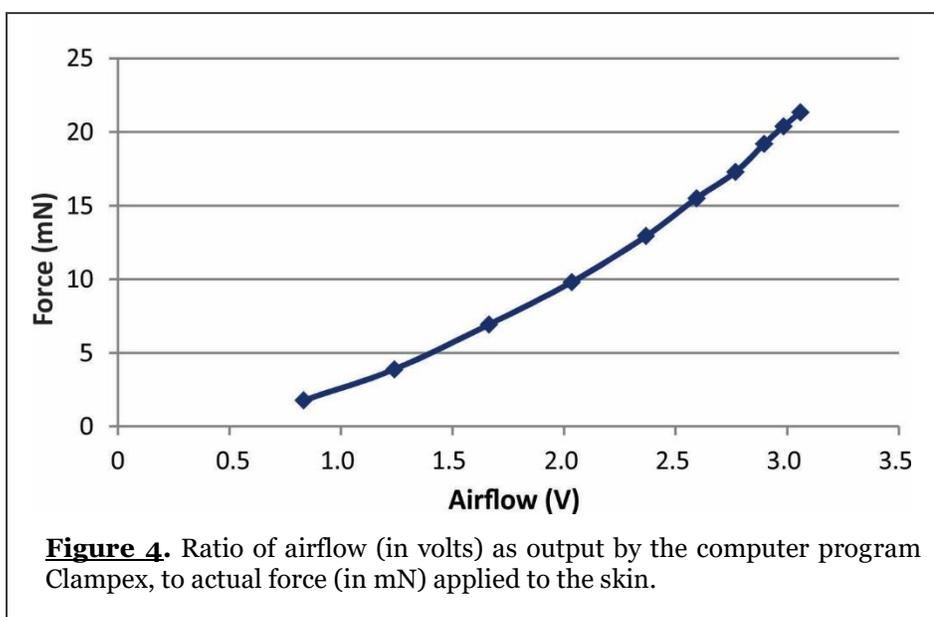
force plate to calibrate the actual amount of force delivered, in mN, compared to the computer readout, in volts (V), (Figure 4).
