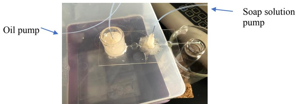
Figure 5 The microfluidic device. The oil comes in one tube, the soap comes in the other and they emulsify and leave into the collecting test tube.
