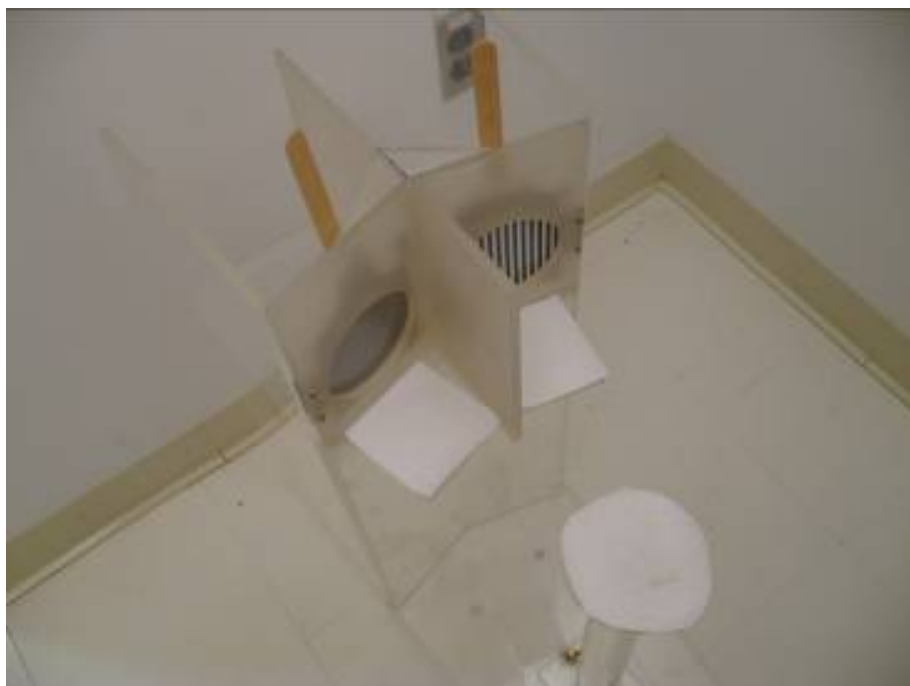
Figure 6. Picture of the acuity apparatus built for the current study. There are no walls, for ease of handling the gerbils. The starting platform is pictured at the correct jumping distance (a gap distance of 15cm). Plexiglass doors containing stimulus cards open outward on hinges, and could be closed shut with a latch in back. The spatial frequency pictured is .6cy/deg from the relevant viewing distance. Shelf liner covered the surfaces to aid in traction.
