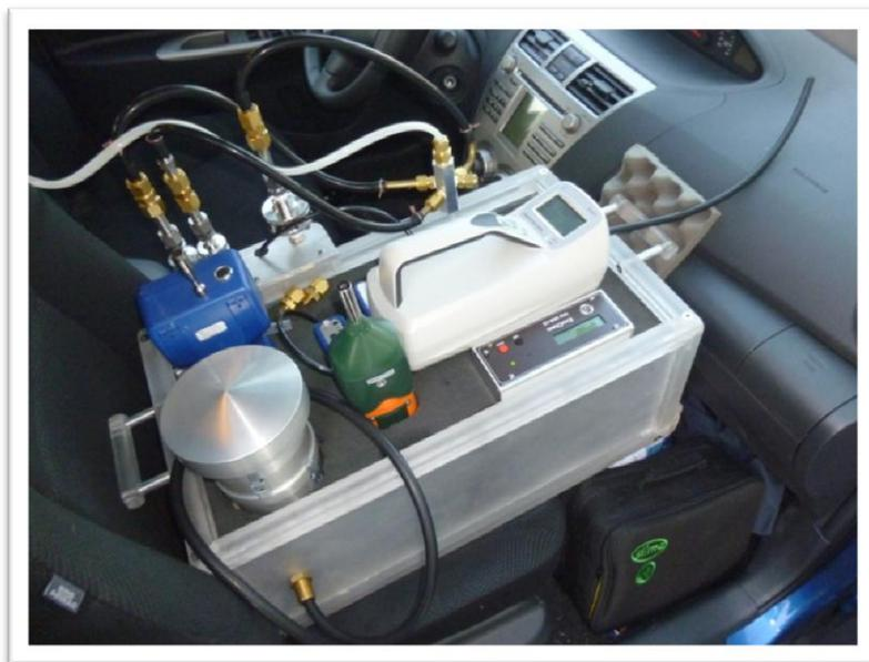
**Figure 1.** A photo of the sampling device manifold containing the exposure sampling devices.
