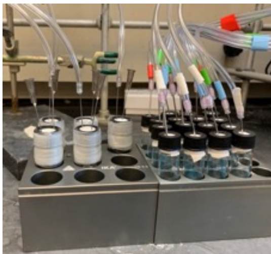
Figure 1. Two of the Blakey Lab dry heating blocks showcasing the ability to run large numbers of reactions efficiently.
