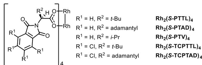
**Figure 1.3** Dirhodium catalysts derived from *N*-phthalimidyl amino acids
