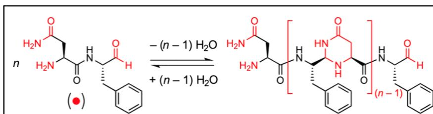
Figure 1. Condensation polymerization scheme of H<sub>2</sub>N-NF-CHO from Chen et al.<sup>4,15</sup>
