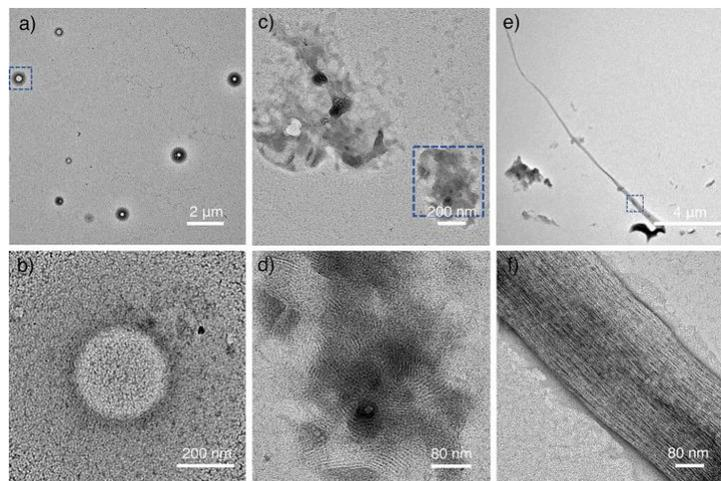
*Figure 10.* TEM Images of NPG system at a) “first few hours”, b) 48 hours, and c) 12 days of assembly in aqueous solution with pH = 4.75 NaOAc/HAc buffer. Data collected by Seth Young and Yushi Bai.<sup>6</sup>
