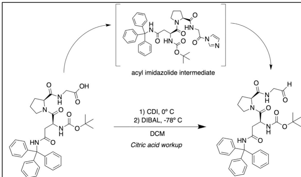
*Figure 3.* Synthetic scheme for reduction of Boc-N(trt)PG-COOH to Boc-N(trt)PG-CHO. Special thanks to Alexis Blake and Alexis Roberson for their hard work in developing and optimizing the process.<sup>21</sup>
