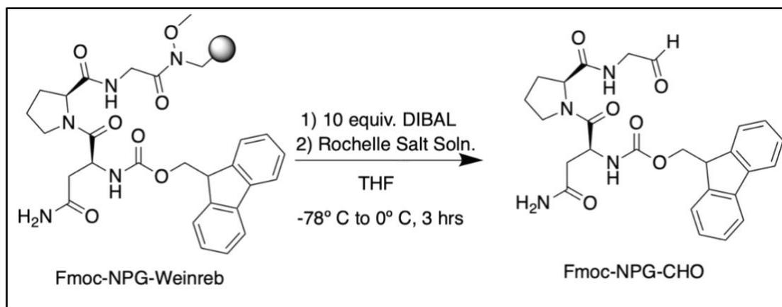
Figure 8. Previously proposed synthetic scheme for reduction to Fmoc-NPG-CHO<sup>16</sup>
