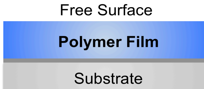
Figure 6. A schematic representation of a supported polymer film. The polymer is fixed to the substrate at the bottom (a silicon wafer with a silicon oxide layer), and exposed to air at the top; these two interfaces can significantly affect the behavior of the polymer.
