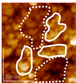
Figure 4.29. AFM image of ATO nanoporous film divided into two kinds of spaces. In the top layer, the regions marked by dotted loop and solid loop were void inter-particle space and filled aggregate space, respectively. The effective filling factors in the two kinds of spaces were different if the inhomogeneity of effective medium approximation existed.
