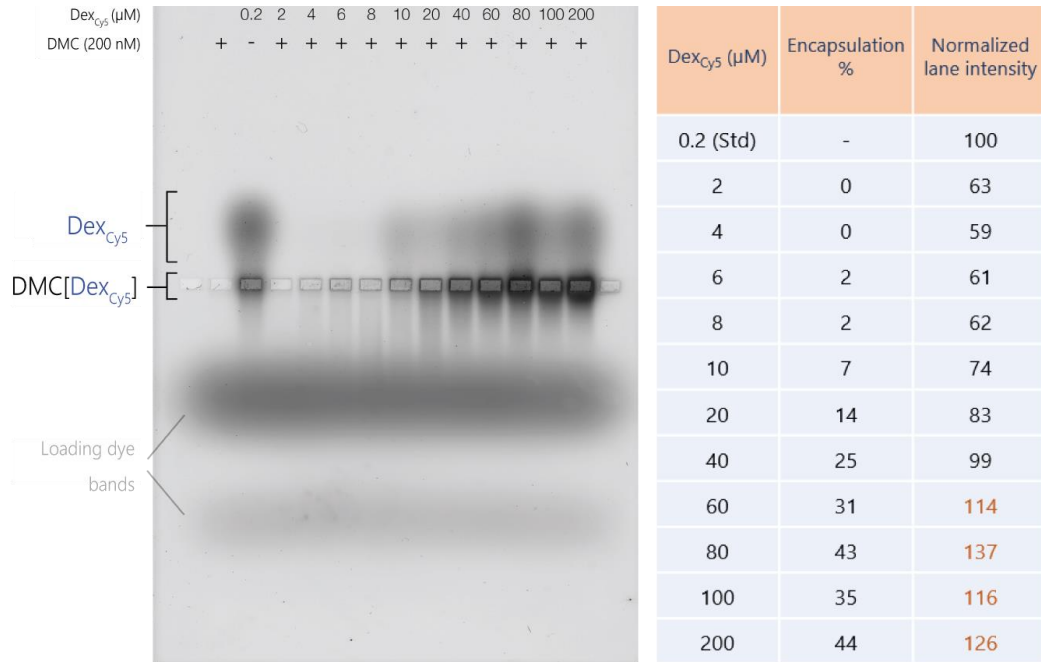
Figure S3 Agarose gel (3.5%) ran with DMC and varying concentrations of Dex Cy5 (Standard concentration - 200 nM Dex Cy5 ). Encapsulation (%) = 100 \times \frac{I_{well}}{I_{standard}} , where I is the integrated intensity of the lane after background subtraction.
