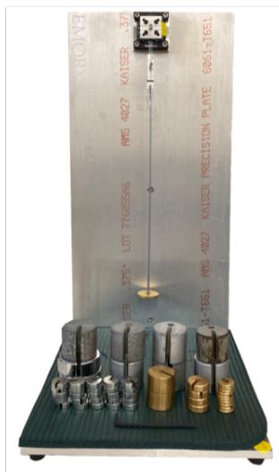
Figure 4.2: Photograph of the CATS Tester along with all of the available masses used for stress-testing. A glass rod sample has been secured to the upper and lower sleeves of the tester.
