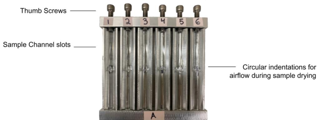
Figure 4.3: Photograph of drying rack used to adhere and dry glass rod samples. Thumb screws at the top of the chamber are used to clamp together ends of the glass rods. The chamber includes circular indentations to encourage airflow during solvent evaporation.
