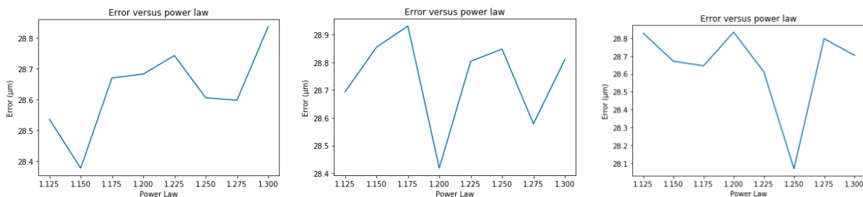
Figure 12. This figure shows the error versus power law graph— where the error is the error in distance with units \mu\text{m} —after running the simulation on each of the varying power laws three times. The minimum values range between 1.15 and 1.25. Therefore, the minimum power law is \beta_f = 1.20 \pm 0.05 .
