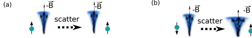
Figure 5.6: (a) Scattering of majority electron by magnetization experiencing only quantum fluctuations. (b) Scattering of minority electron by magnetization enhance quantum fluctuations.
