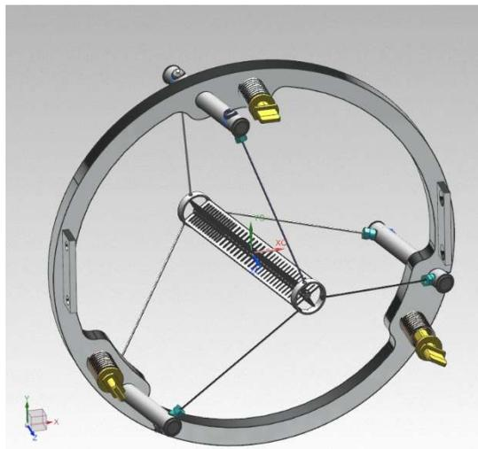
**Figure 1.10:** Bicycle wheel mount for the production target [8].
