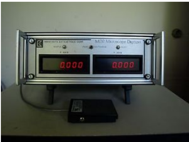
Figure 5: Stereological setup. The sampling grid and counting frame laid on the computer monitor showing the layers of cortex (Layer IIIA is yellow line to blue dotted line). As the microscope slide stage was moved, spatial information was sent to the Minnesota Datametrics hardware and ultimately virtually represented on screen. This setup allowed for systematic, random sampling of the region of interest.
