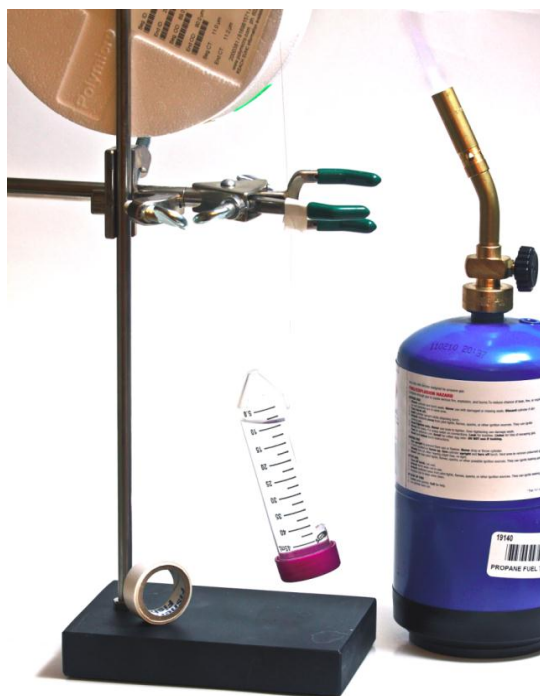
Figure 6. Pulling of the inner capillary. The inner capillary is attached to a conical tube containing 45 mL of water and is then placed onto a support stand. The tube pulls the capillary, which is melted with a propane pencil flame burner.
