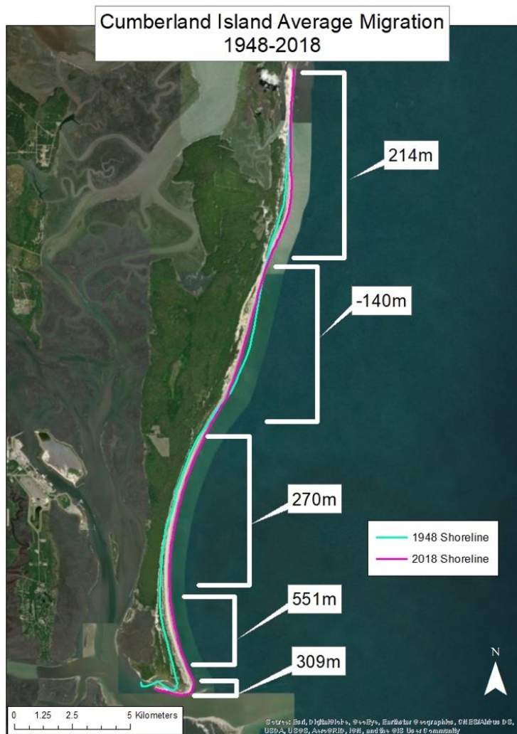
Figure 4. Shoreline accretion or erosion of different sections of Cumberland Island between 1948 and 2018.
