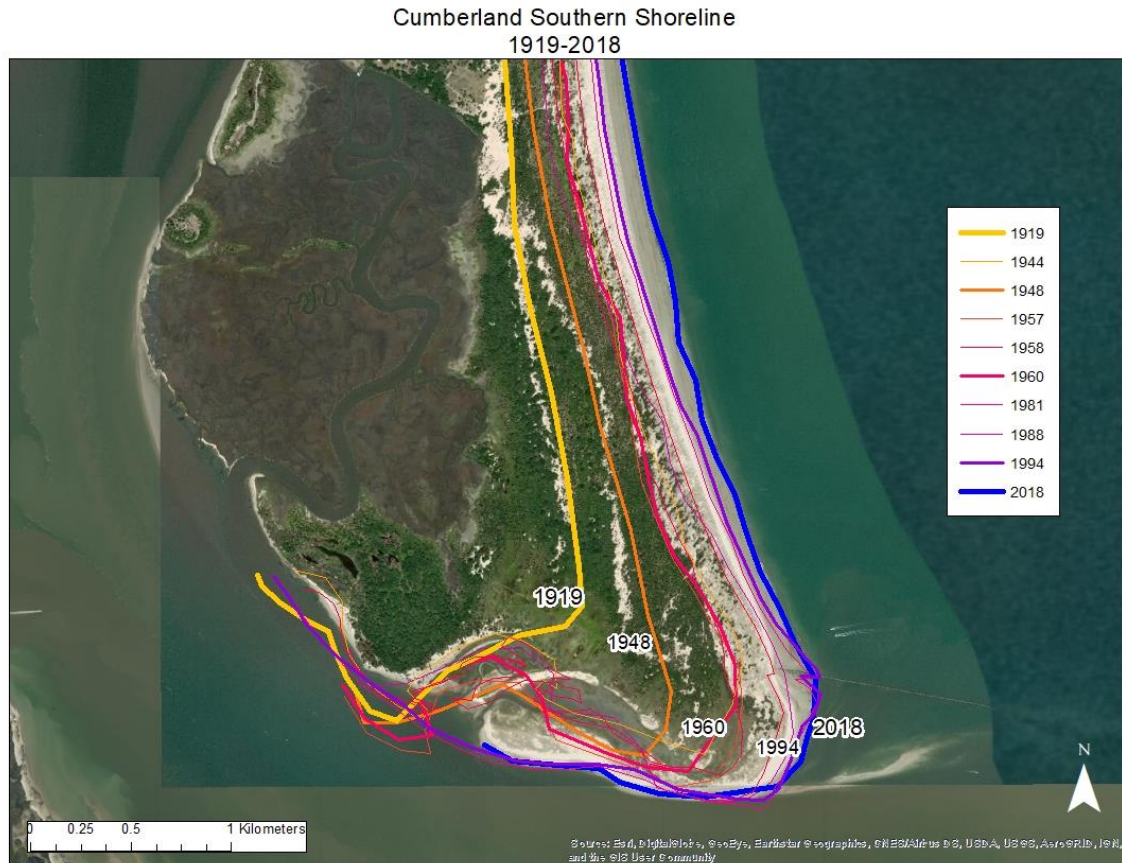
Figure 5. Shoreline changes discerned from topographic maps of southern end of Cumberland Island. The shoreline accreted at a normal rate north of the jetty, but halted south of the jetty.
