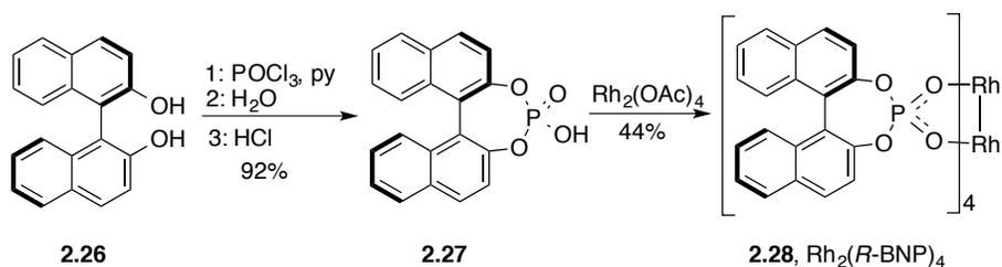
**Scheme 2.7** The synthetic route of Rh<sub>2</sub>(R-BNP)<sub>4</sub>
