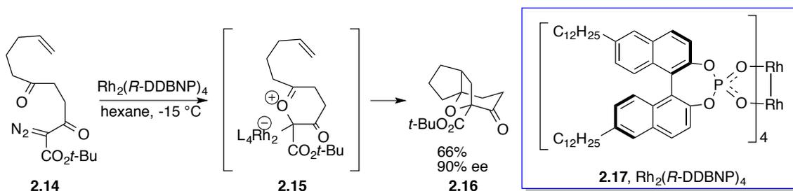
**Scheme 2.3**  $\text{Rh}_2(\text{R-DDBNP})_4$ -catalyzed 1,3-dipolar cycloaddition
