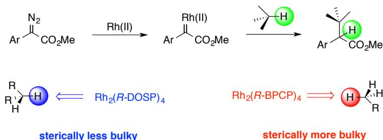
**Scheme 7.1** Concept of catalyst-controlled site selective C–H functionalization
