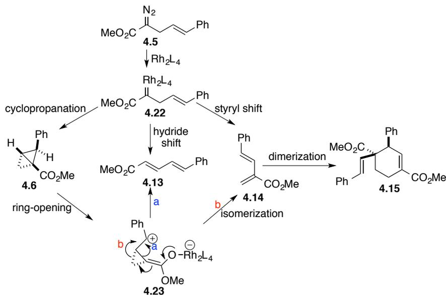
Scheme 4.8 Proposed possible mechanism for cyclohexene formation
