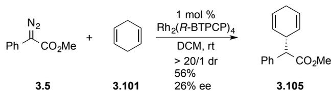
**Scheme 3.18**  $\text{Rh}_2(\text{R-BTPCP})_4$ -catalyzed C–H insertion with phenyl diazoacetate
