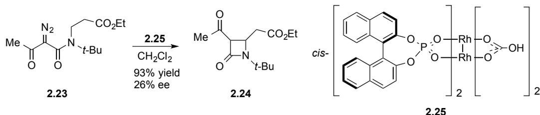
**Scheme 2.6**  $\text{Rh}_2(\text{S-BNP})_2(\text{HCO}_3)_2$ -catalyzed intramolecular C–H insertion
