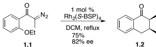
**Scheme 1.1**  $\text{Rh}_2(\text{S-BSP})_4$ -catalyzed intramolecular C–H insertion reaction
