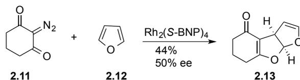
**Scheme 2.2**  $\text{Rh}_2(\text{S-BNP})_4$ -catalyzed reaction with furan
