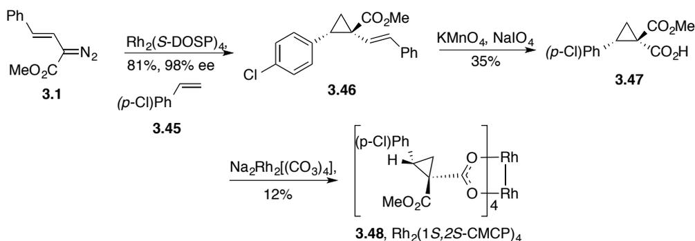
**Scheme 3.11** The synthetic routes towards Rh<sub>2</sub>(1*S*,2*S*-CMCP)<sub>4</sub>
