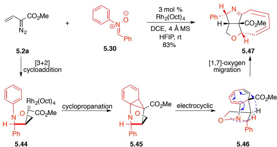
**Scheme 5.10** The Doyle's cascade reaction with nitron
