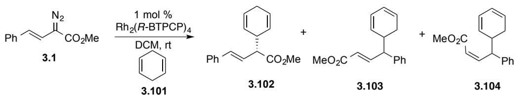
**Scheme 3.17**  $\text{Rh}_2(\text{R-BTPCP})_4$ -catalyzed C–H insertion with styryl diazoacetate
