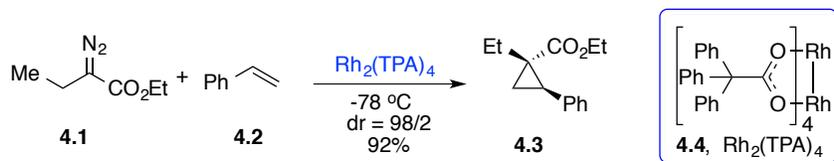
**Scheme 4.1** Inhibiting  $\beta$ -hydride shift from metallocarbene with bulky  $\text{Rh}_2(\text{TPA})_4$
