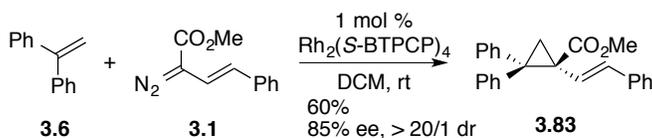
**Scheme 3.12** Rh<sub>2</sub>(*S*-BTPCP)<sub>4</sub>-catalyzed cyclopropanation of 1,1-diphenylethylene
