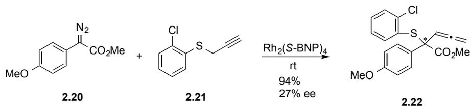
**Scheme 2.5**  $\text{Rh}_2(\text{S-BNP})_4$ -catalyzed [2,3]-sigmatropic rearrangement
