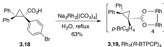
**Scheme 3.8** The synthesis of Rh<sub>2</sub>(*R*-BTPCP)<sub>4</sub> catalyst
