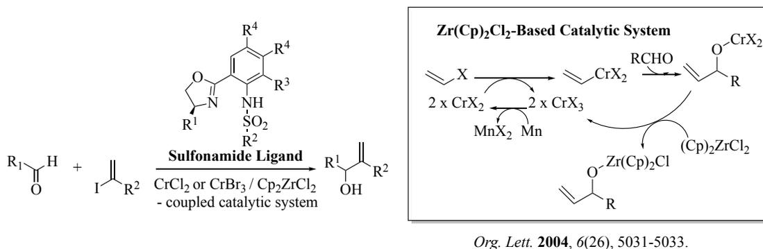
**Figure 15.** Zirconocene dichloride (Cp<sub>2</sub>ZrCl<sub>2</sub>) for Cr-mediated Nozaki-Hiyama-Kishi coupling of aldehydes with halides.
