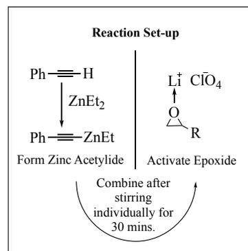
**Figure 17.** Progression of reaction with benzyl glycidyl ether **40** and phenylacetylene **17** using lithium perchlorate ( $\text{LiClO}_4$ ) and diethylzinc.
