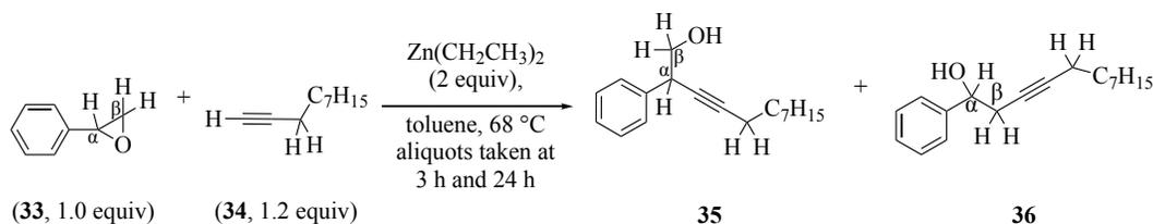
Under an argon balloon, a solution of  $\text{ZnEt}_2$  (0.450 mL, 1.0 M in hexane, 0.450 mmol, 2.0 equiv) was added to cooled, anhydrous toluene (0.35 mL). The mixture was stirred at room temperature for 30 min. 1-decyne **34** (0.048 mL, 0.27 mmol, 1.2 equiv) was then added dropwise and stirred
