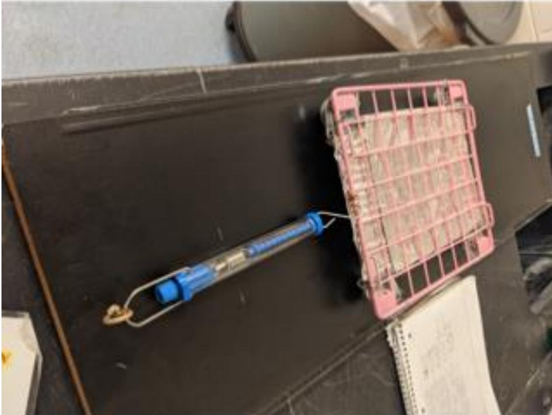
Figure 16: Homemade (old) Grip Strength Meter.
