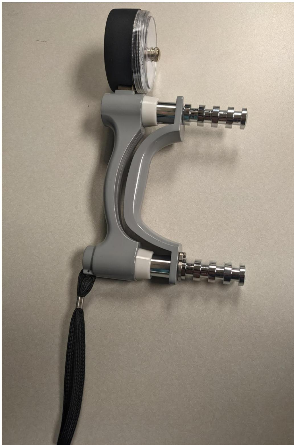
Figure 2: Jamar Hand Dynamometer.
