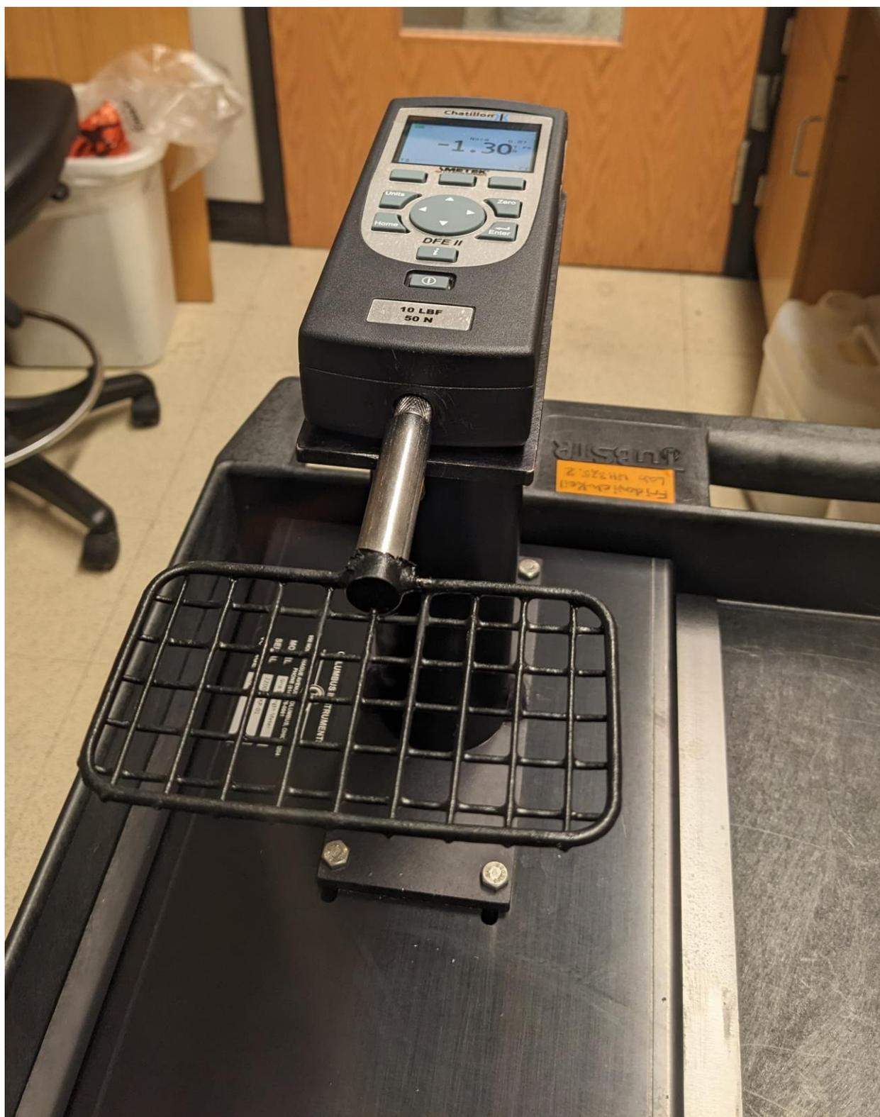
Figure 17: Columbus Instruments (new) Grip Strength Meter
