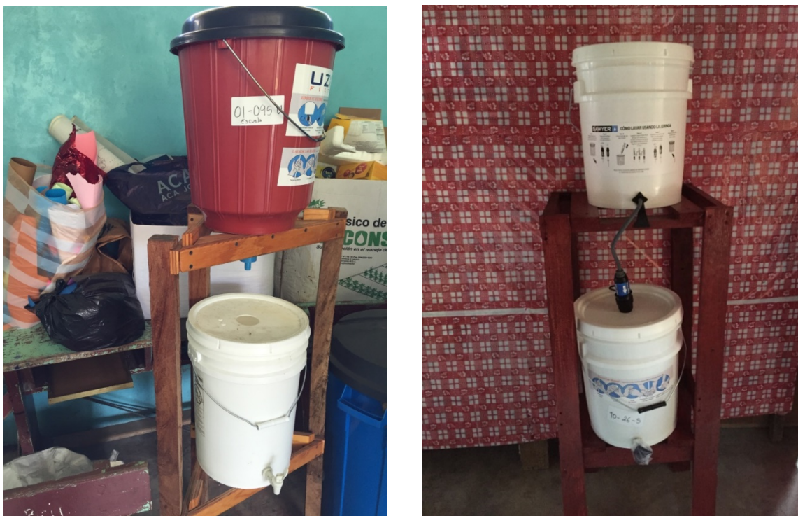
Figure 2 Uzima (on left) & Sawyer (on right) filters on wooden stands in project households in the evaluation of a hollow fiber membrane filtration program in the Agalta Valley, Honduras, January-July 2016 (Reproduced with permission from Sera Global Health Practice)
