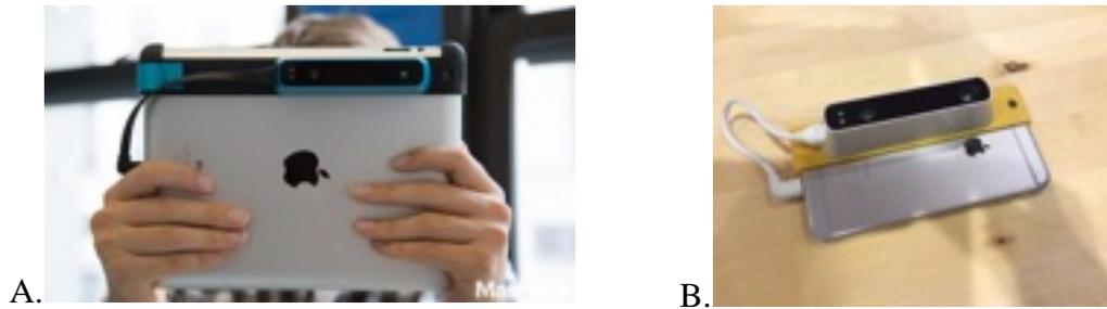
Figure 2-1 A. Hardware setup for the Body Imaging for Nutritional Assessment Study — Structure Sensor connected to tablet. B. Structure Sensor connected to mobile phone
