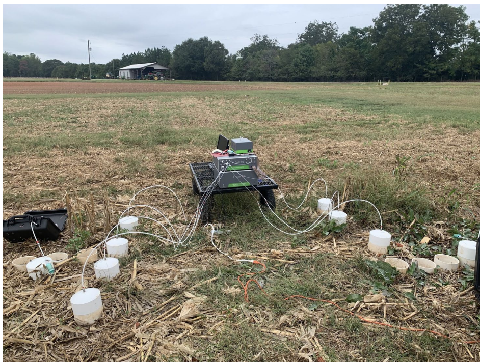
Figure 1: Closed chambers connected to Picarro during concentration collection.
