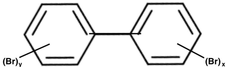
**Figure 2: General structure of PCBs**
