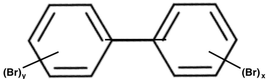
**Figure 2: General structure of PCBs**
