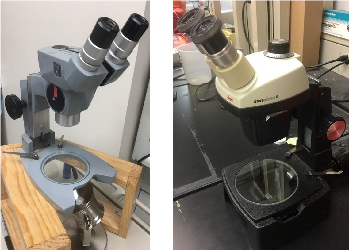
**Figure 1. Examples of stereo microscopes with oblique illumination that can be used to visualize colony opacity.** Two separate microscopes that are used in our lab to visualize differences in colony opacity. It is essential to have a light source with an angle that can be adjusted to visualize the colony opacity phenotypes.
