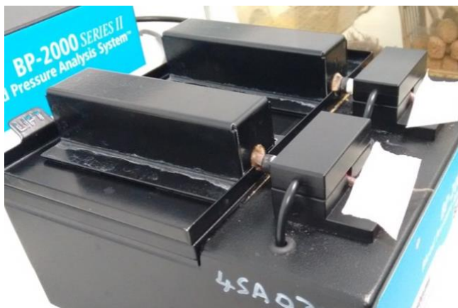
Figure 7: Apparatus of Visitech BP-2000 tail cuff system. Mice are placed on a heated platform which prevents thermal vasoconstriction, and their tails are taped to minimize excessive movement. Image acquired from
