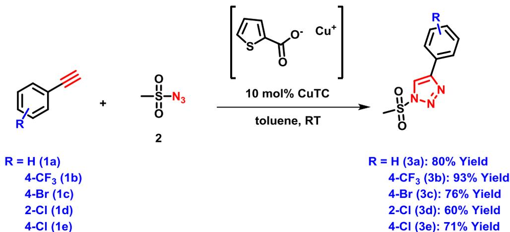
**Scheme 3.2.** Synthesis of 1-*N*-sulfonyl-1,2,3-triazole derivatives
