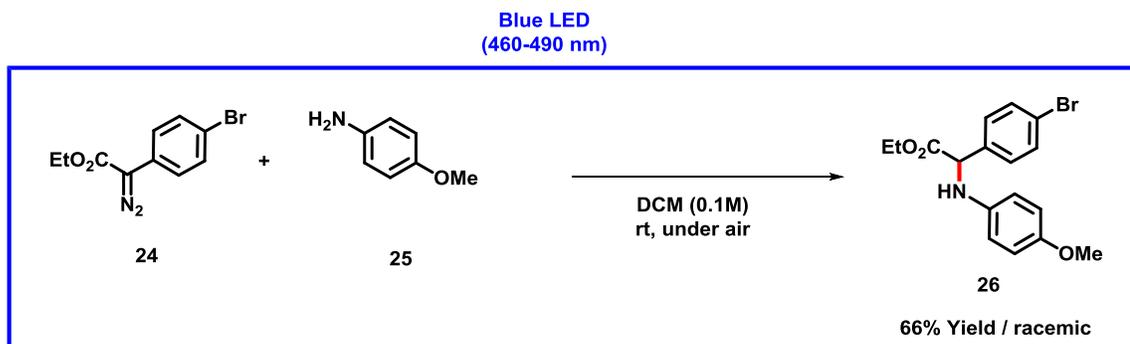
**Scheme 2.12.** N-H insertion reaction with blue LED as photochemistry
