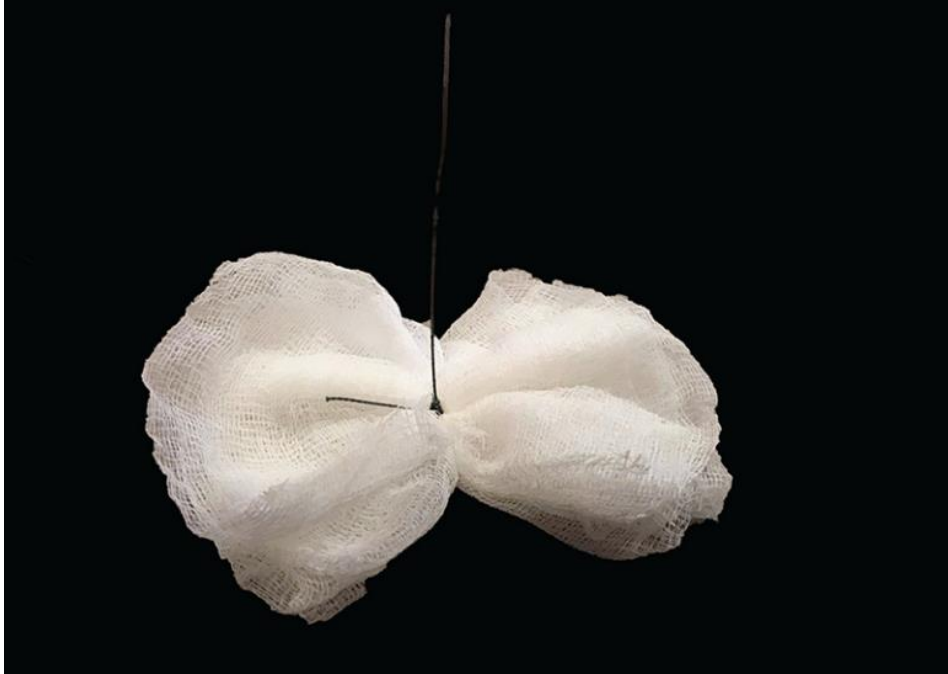
Figure 5 displays the Moore Swab used by the Moe Research Team for wastewater surveillance sampling. Figure provided by Moe Research Team.
