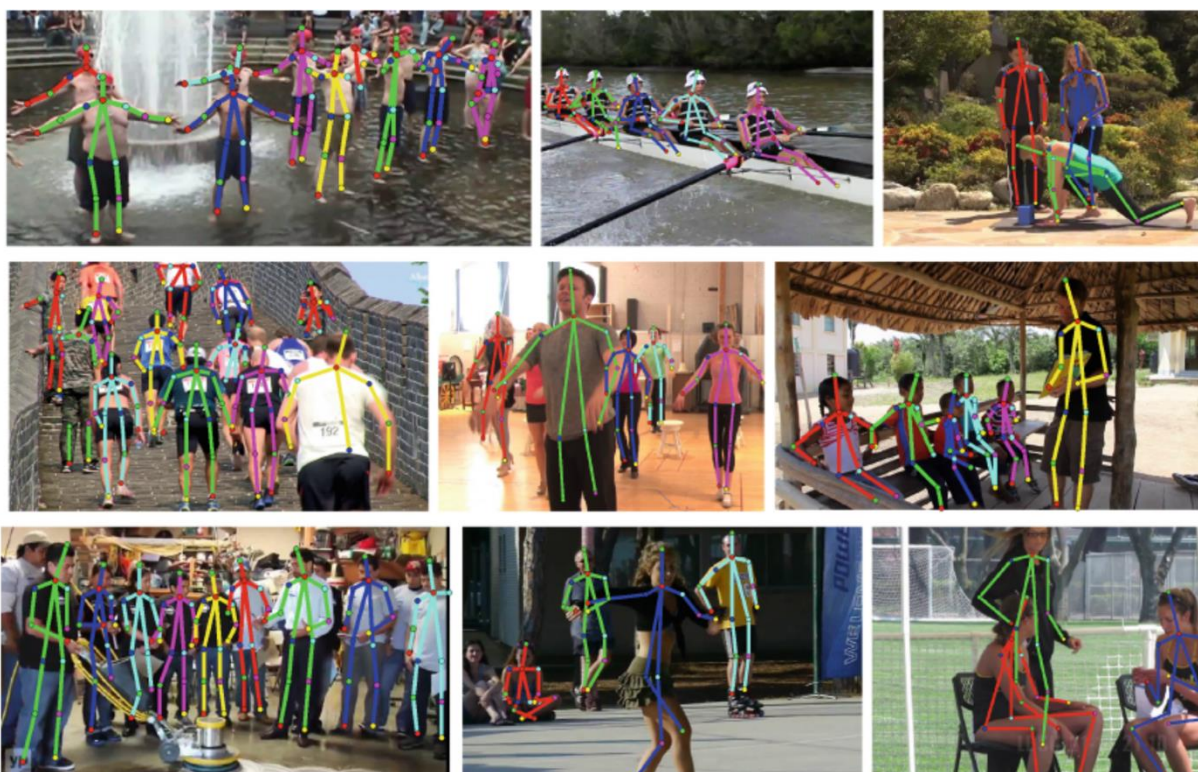
Figure 3.3. An example illustrating an application of deep-learning tools for human pose estimation of multiple people in real-world images. (Adapted from Insafutdinov et al., 2016)
