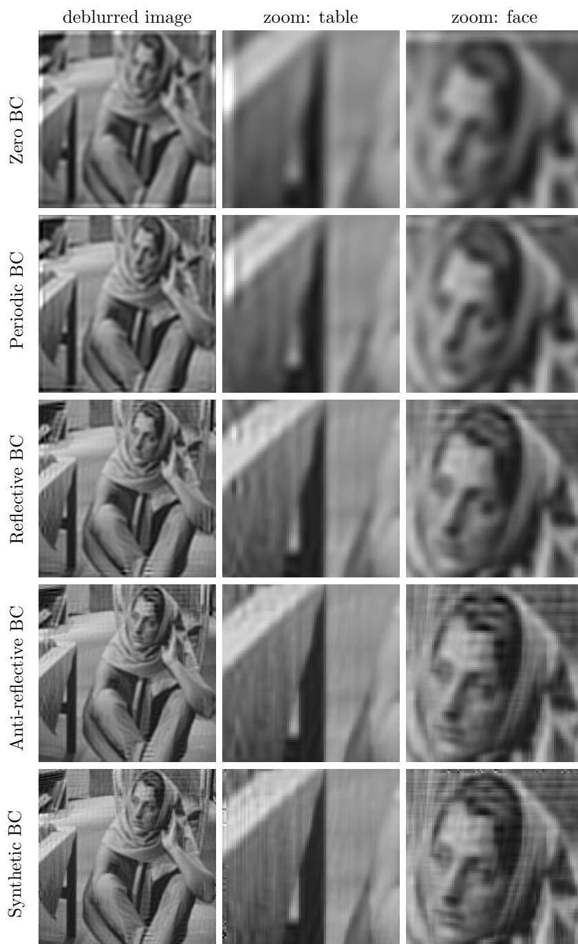
Figure 2.6: Deblurring results on Gaussian blurred “Barbara” with different boundary conditions
