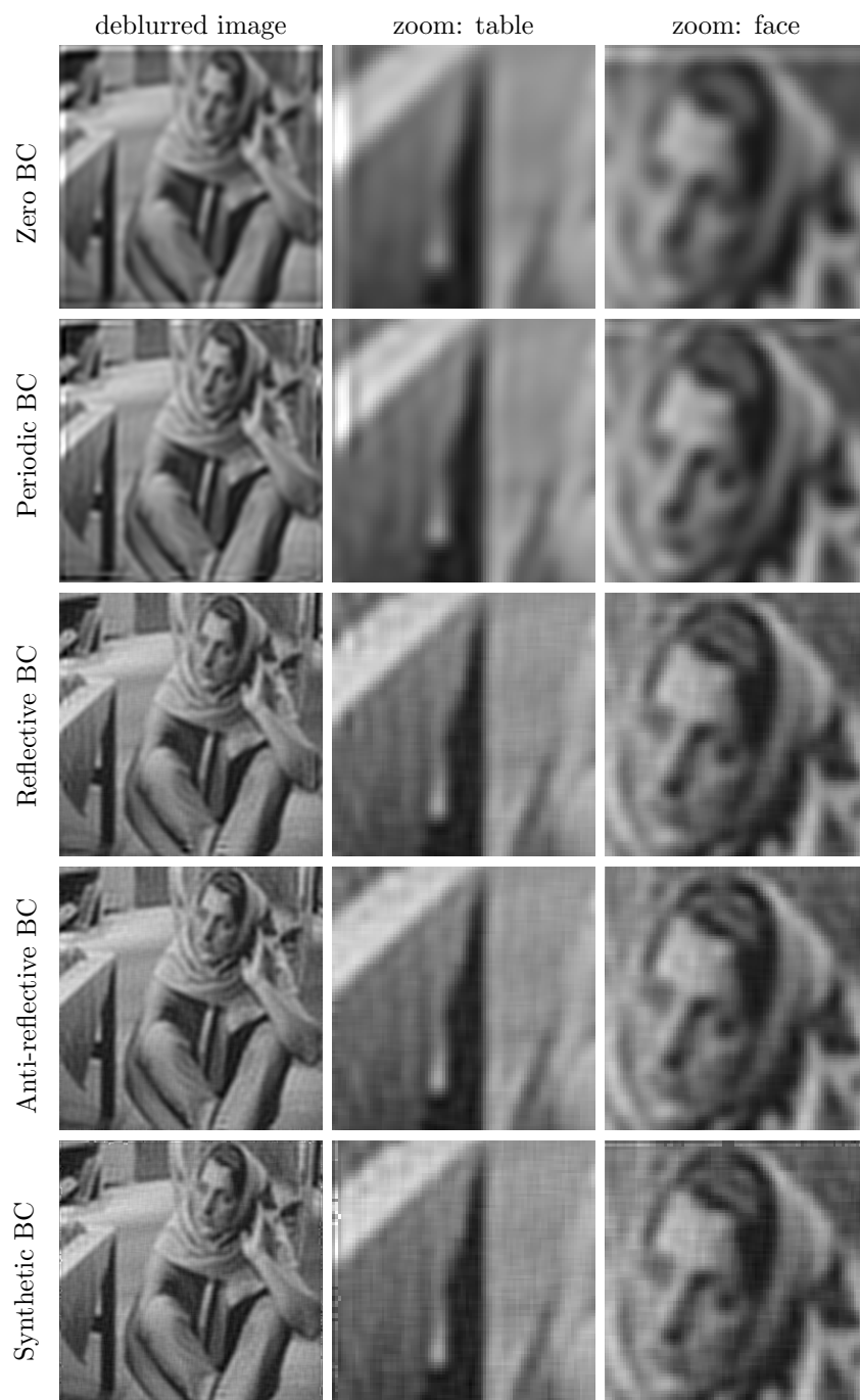
Figure 2.11: Deblurring results on noisy Gaussian blurred “Barbara” with different boundary conditions
