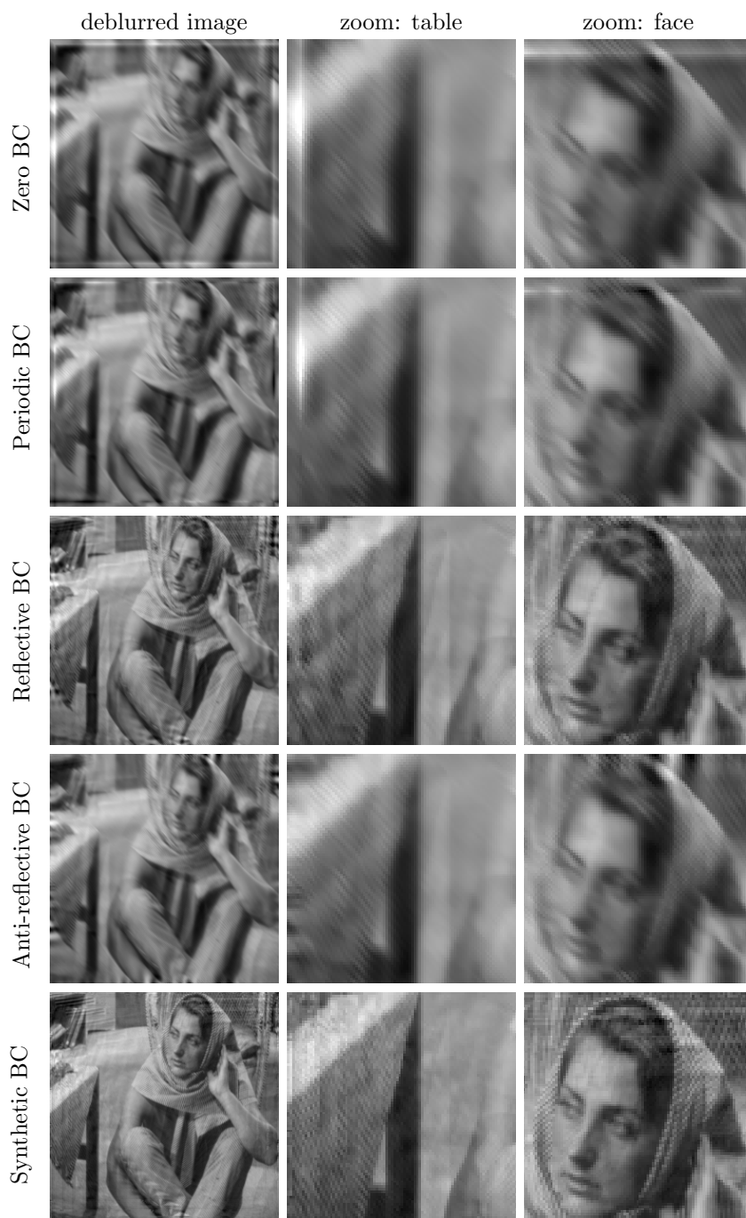
Figure 2.9: Deblurring results on motion blurred “Barbara” with different boundary conditions
