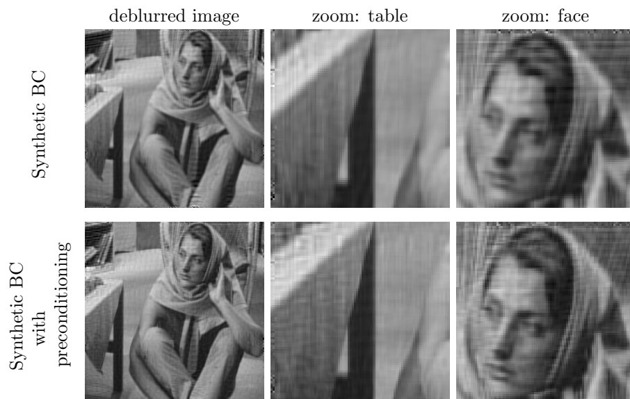
Figure 2.17: Deblurring results on Gaussian blurred “Barbara” with synthetic boundary conditions. The first row is obtained without preconditioning at the 500th iteration; the second row is obtained with preconditioning at the 20th iteration.
