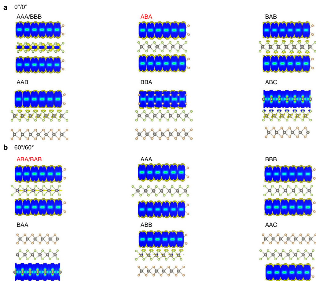
Figure E11. DFT calculation of electron distribution for AA stacked samples. a. Electron distribution in 0^\circ/0^\circ samples. b. Electron distribution in 60^\circ/60^\circ samples. The red highlighted ABA in 0^\circ/0^\circ and ABA/BAB in 60^\circ/60^\circ are the lowest energy states.
