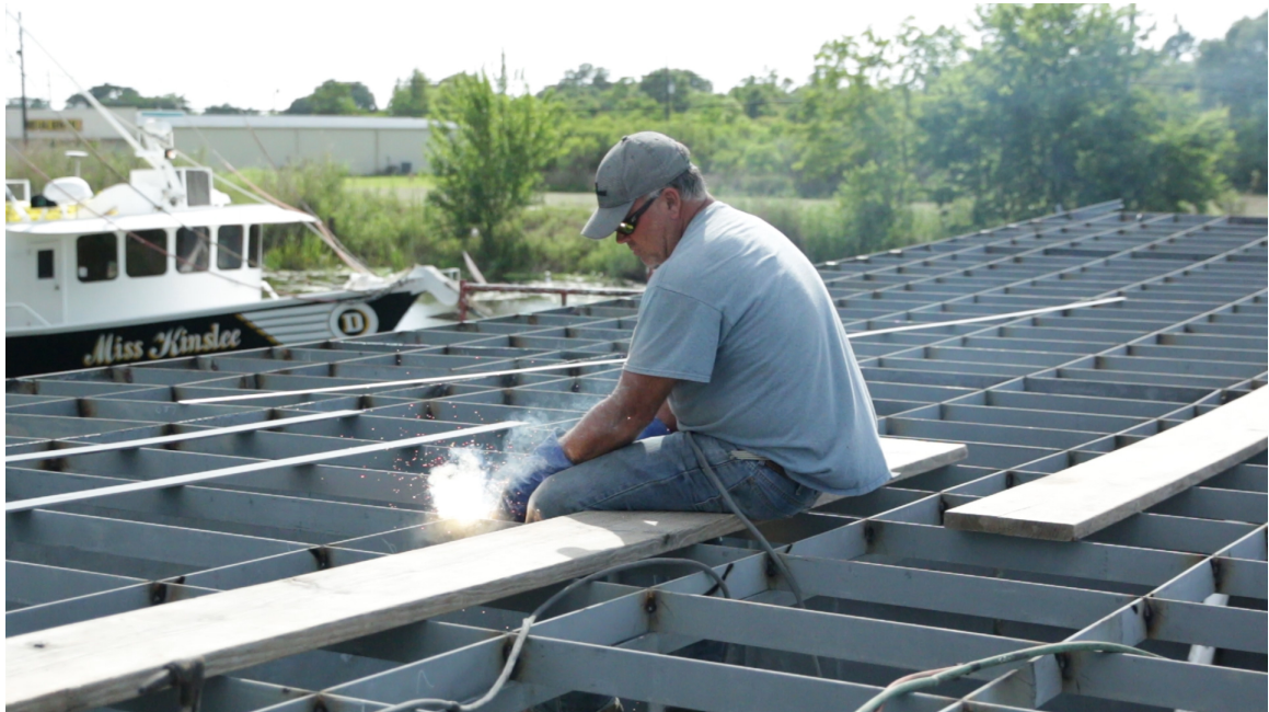
Figure 26: Chad Portier welding together the steel frame of a shrimp boat. Photograph by Christopher Lirette.
