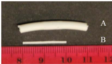
Figure 5. A) Our old needle made from a magnetic stir bar in plastic tubing. It is covered in Teflon tape to increase the surface tension between it and water. The size difference and curvature of the old needle are clearly visible. It is 3.65 mm thick. B) Our new needle made of rolled steel. We covered it the top surface in white tape to make imaging it easier. It is .2 mm thick.
