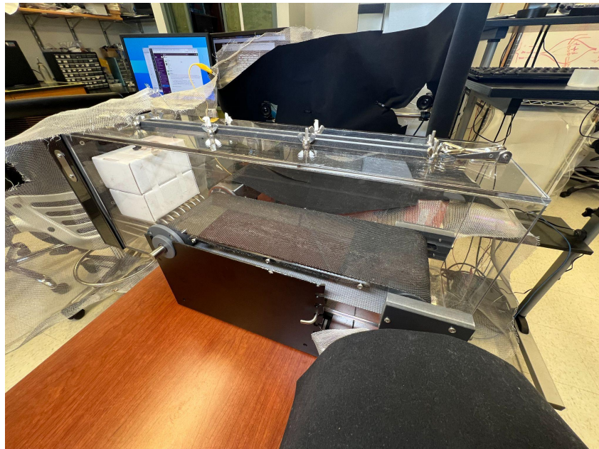
Figure 2. Rat locomotion training treadmill set at incline 0.
