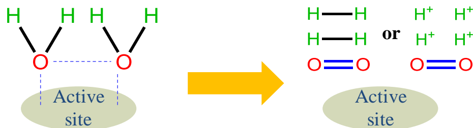
Figure 1.6. Schematic representation of water splitting catalyzed by an active site.
