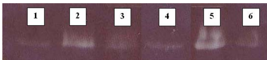
Figure 2.7 SDS-PAGE gel of MAO samples exposed under UV light. (1) human MAO A, (2) DCP-inhibited MAO A, (3) clorgyline-inhibited MAO A with DCP (1:1), (4) human MAO B, (5) DCP-inhibited MAO B, and (6) pargyline-inhibited MAO B with DCP (1:1).
