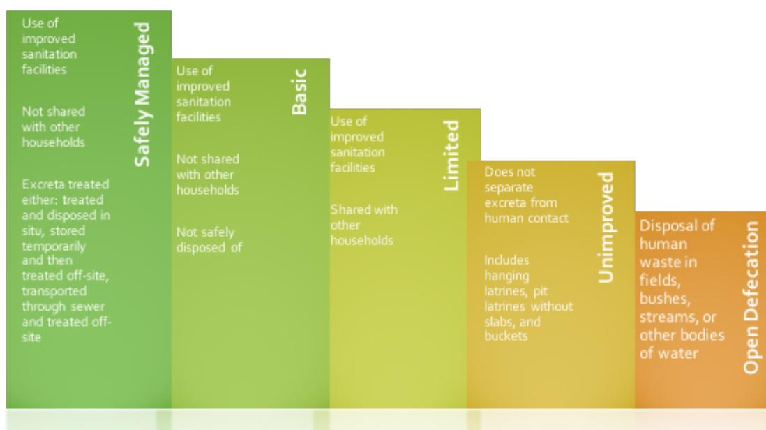
Figure 2: JMP Service Ladder for Sanitation 29 . This ‘sanitation ladder’ is an update to the MDG sanitation ladder (see Figure 1) for the new Sustainable Development Goal (SDG) era WASH goals. The previous category of “improved” has been subdivided, leading to five ‘rungs’ in the ladder, rather than the previous 4. Adapted from JMP 29
