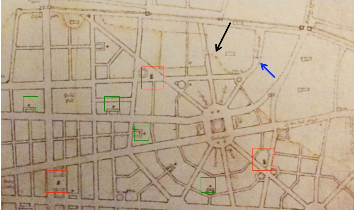
Figure 5. Wren labeling system used in his plan for rebuilding London. Black arrow pointing at dashed line representing extent of the fire damage. Blue arrow pointing at dotted line representing existing roads. Red boxes contain the symbol of mercury demarcating markets. Green boxes have small crosses delineating the location of churches.
