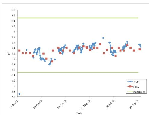
Figure 30 – Comparison of pH monitored by remote sensor (AMS) to measurements on discrete grab samples (COA), with regulations WTP, 2012
