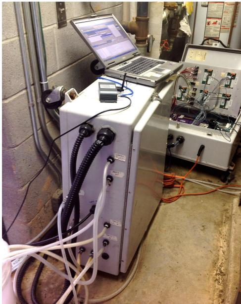
Figure 39 – AMS controller box, probe box, and laptop inside Fire Station field site #2
