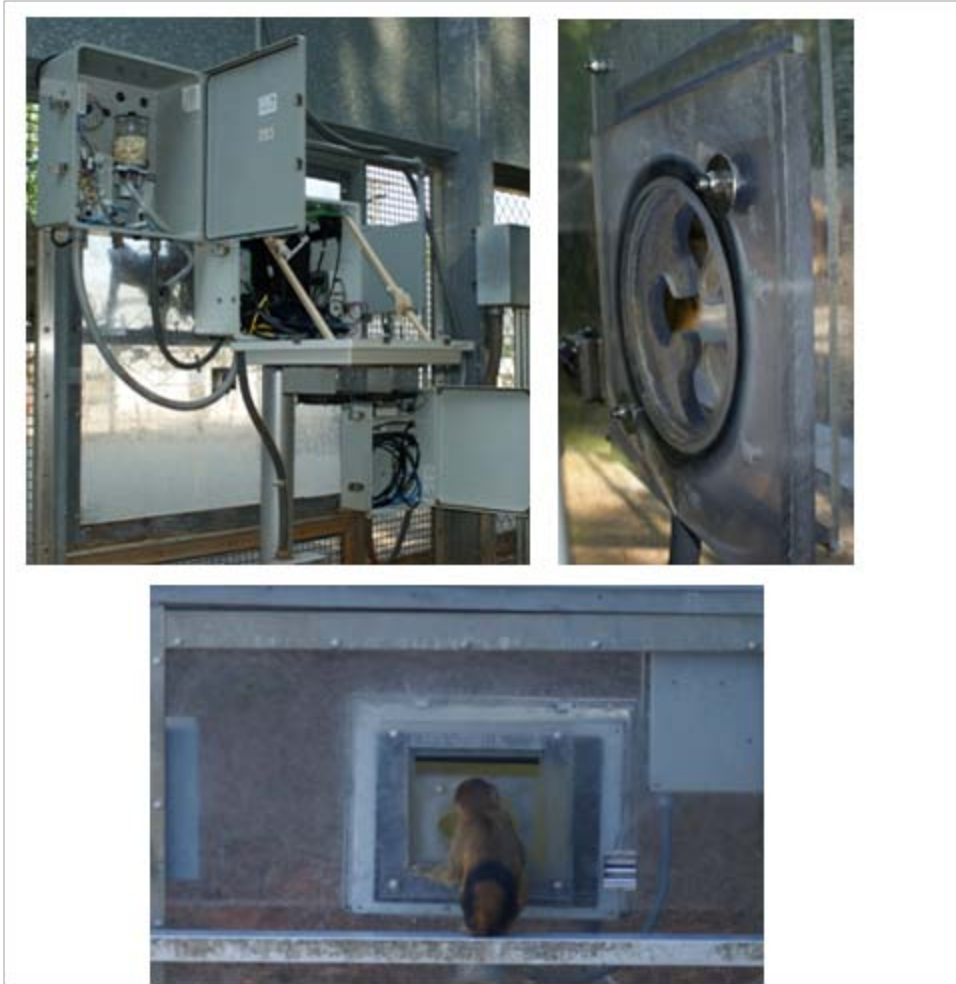
Figure 2: Kiosk components. Top left: viewed from just outside the monkey social group, all weatherproof boxes housing kiosk components, including the pellet dispenser and reader, touch screen and netbook, and related components. Top right: armhole encircled by the RFID antenna (black). Bottom: the kiosk from the monkey's perspective inside the compound.
