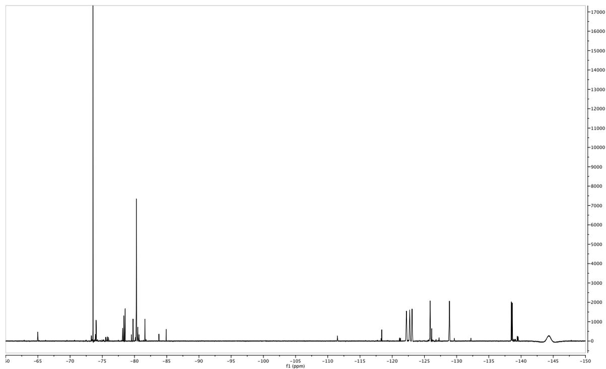
**Figure 5.4**  $^{19}\text{F}$  NMR of PFOA Degradation Products (DMSO:MeCN, 100 °C, 8 hours)
