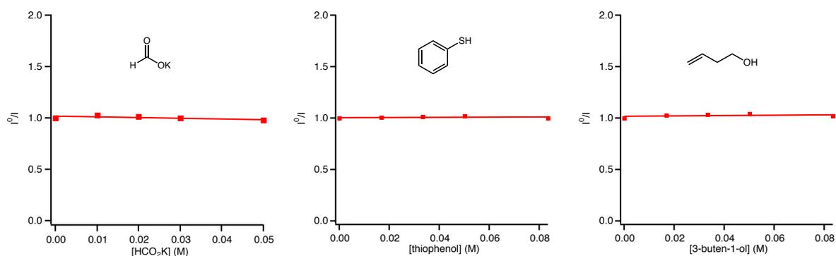
**Figure 4.8** Stern Volmer Plots of Other Reaction Components
