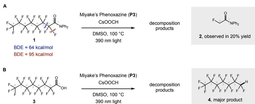
**Figure 5.2** Controlled decomposition and characterization of PFAS using photoredox
