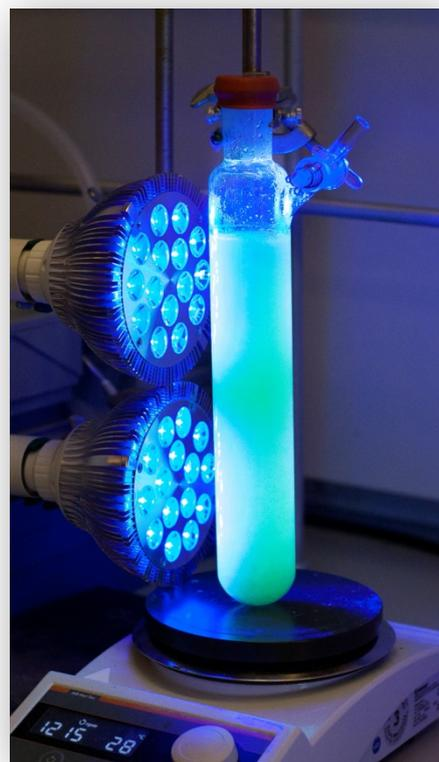
**Figure 1.4** Limited light penetration of large scale photoredox reactions
