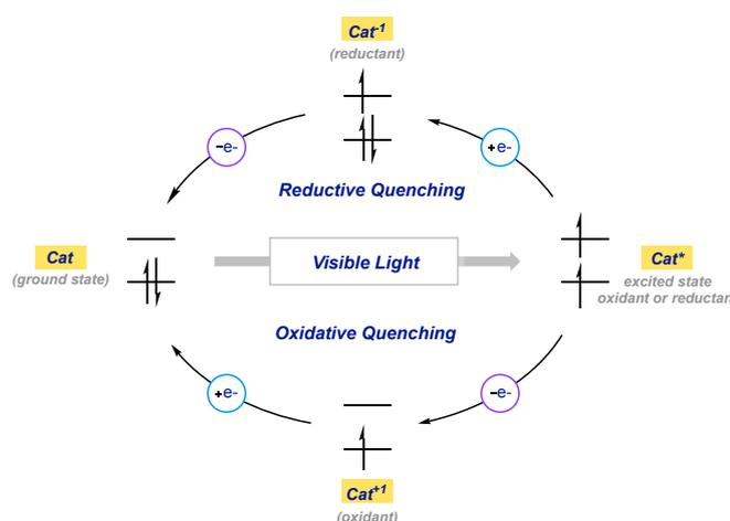
**Figure 1.2** Outer Sphere Electron Transfer Mechanisms
