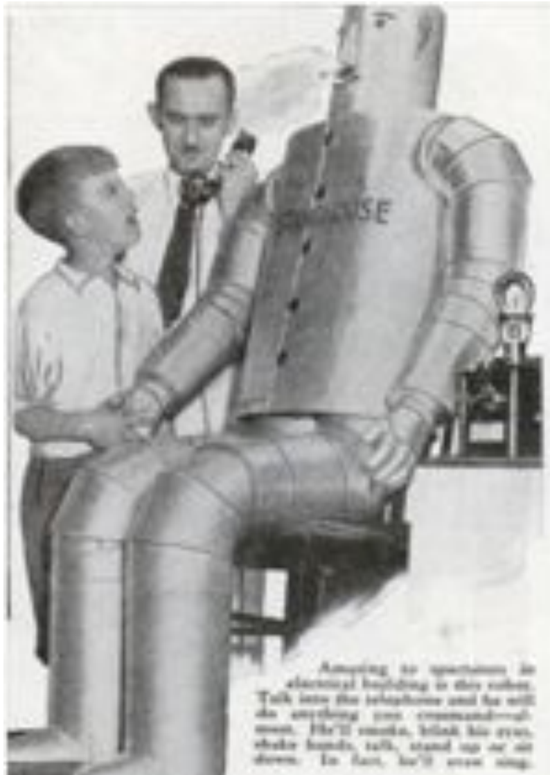
Detail from "Chicago World's Fair" article in Modern Mechanix , October 1933, 73. Here J.M. Barnett gives Willie instructions via a telephone. His verbal commands are transferred by photoelectric cells to the control system, a modified Televox unit. 121
