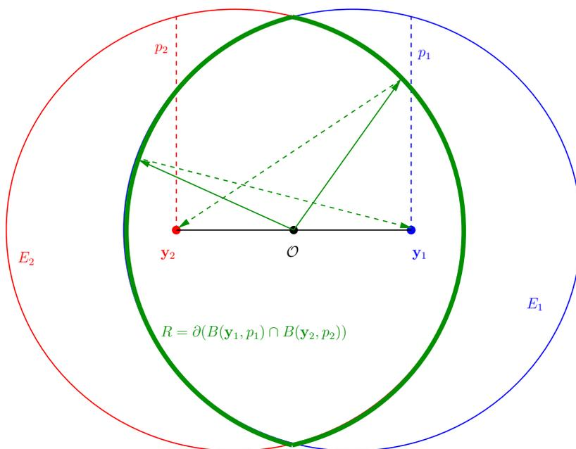
Figure 3.1: The reflector  $R$  generated by the ellipses  $E_1 = E(\mathbf{y}_1, 4a)$  and  $E_2 = E(\mathbf{y}_2, 4a)$  redistributes the light emitted from a homogeneous source evenly among the target points  $\mathbf{y}_1$  and  $\mathbf{y}_2$ .
