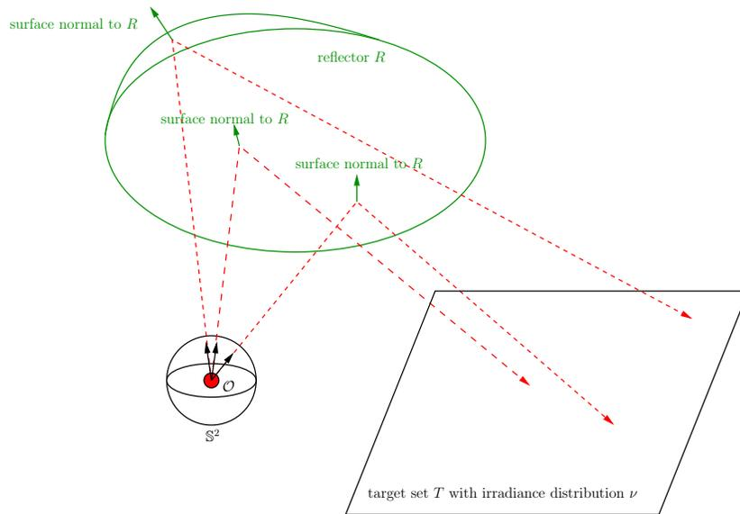
Figure 1.1: An illustration of the near-field reflector problem in  $\mathbb{R}^3$ . The radiation intensity of the point source at the origin  $\mathcal{O}$  is given by a non-negative function  $I \in L^1(\mathbb{S}^2)$ . The design problem consists of finding the reflector  $R$  such that the reflected rays produce the prescribed irradiance distribution on the target set which is given by a Borel measure  $\nu$ .
