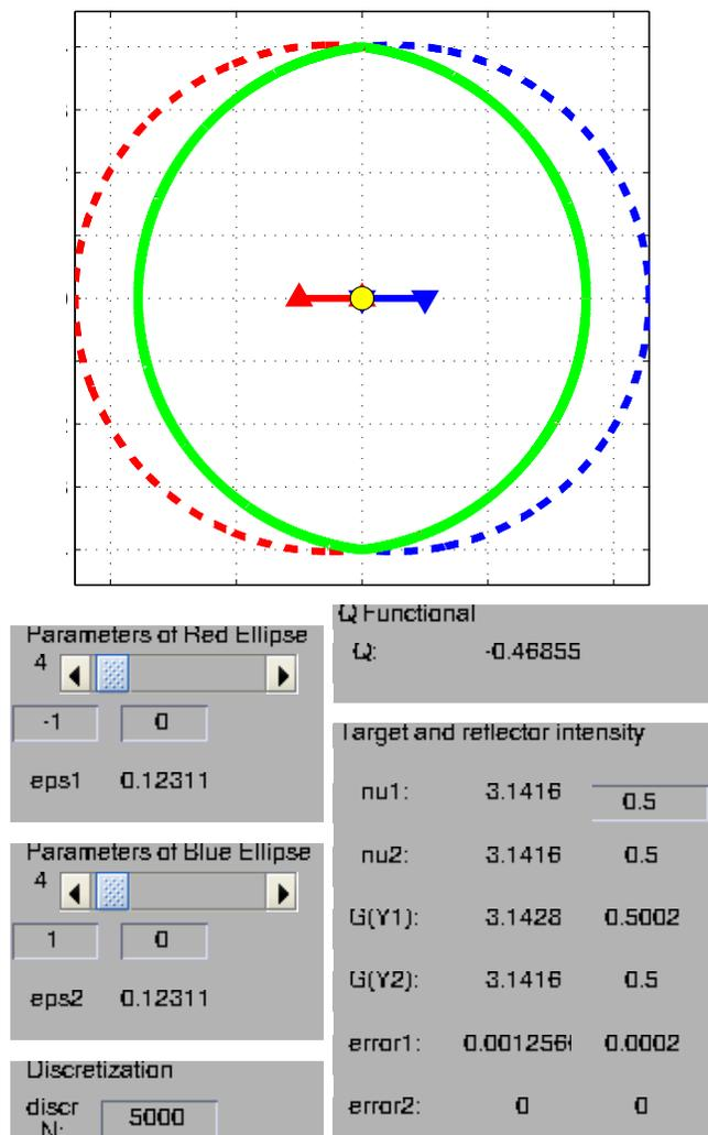
Figure 3.2: The solution to the reflector problem (3.11) and the corresponding GUI panels. Top: display panel, bottom left: control panel, bottom right: output panel
