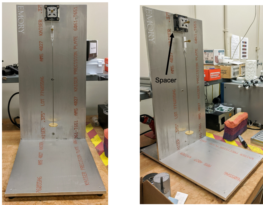
Figure 6.8: Two views of the completed testing device. The supports on the back have been changed to one larger support, and an extra spacer has been placed between the rotation stage and the back board.
