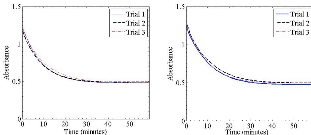
**Figure 8.** Reaction of photo-generated cob(I)inamide in aqueous solution at pH 6.0. Left: Water was added to the sample, as a control for the addition of bicarbonate solution. Right: No additions to the sample. The absorbance was detected at 387 nm, which corresponds to the UV absorption peak of cob(I)inamide.
