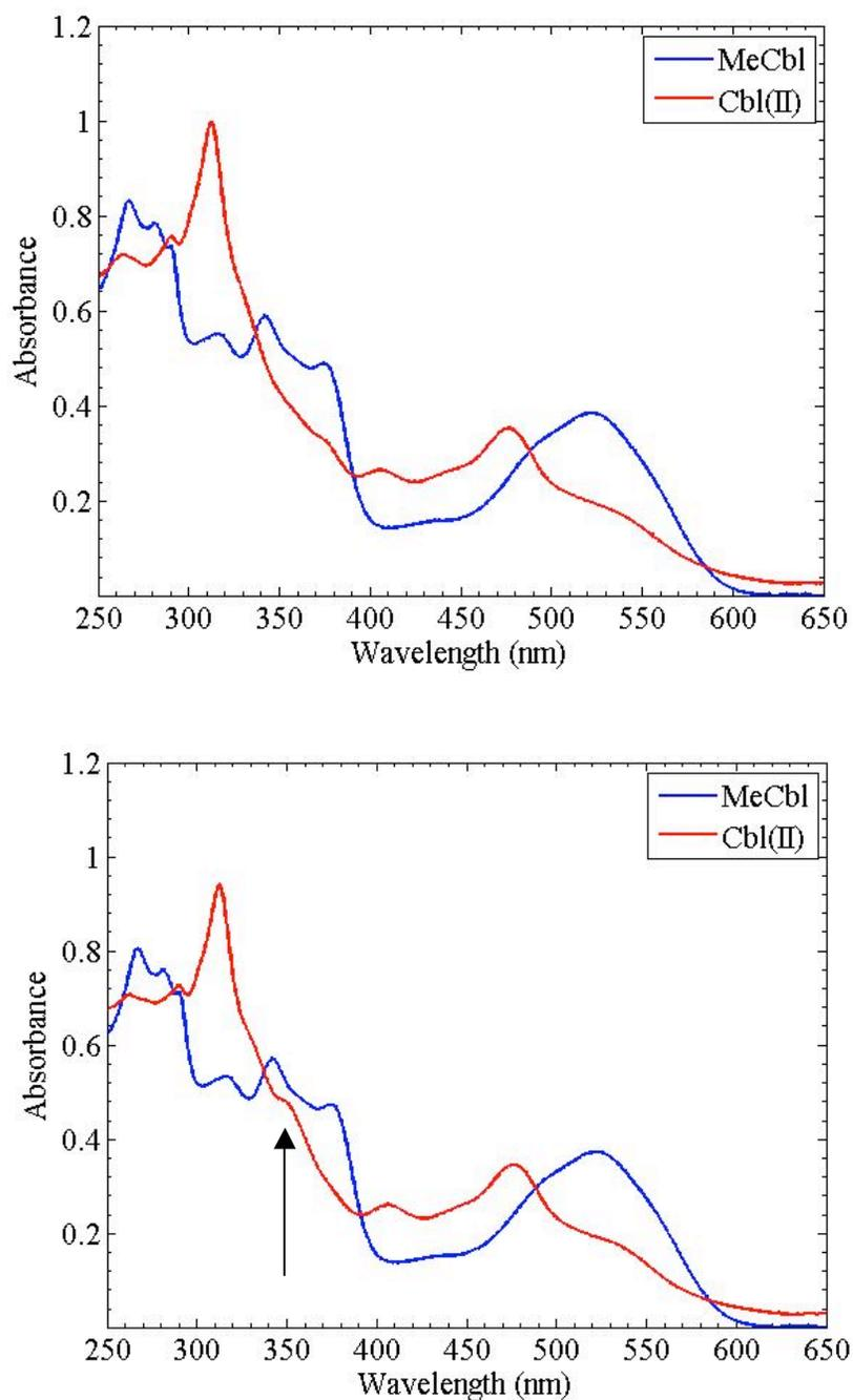
**Figure 7.** (Above) Ultraviolet/visible spectra of MeCbl and photolysis to Cbl(II) without bicarbonate added, (Below) Ultraviolet/visible spectra of MeCbl and photolysis to Cbl(II) with bicarbonate added
