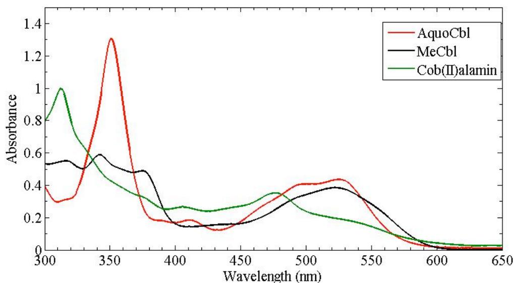
**Figure 5.** UV/visible absorption spectra of cobalamin compounds in aqueous solution at room temperature. The cobalamin concentrations are  $50 \mu\text{M}$ , in  $10 \text{ mM}$  MES, pH 6.0 (MeCbl and cob(II)alamin) and pure water (AquoCbl).
