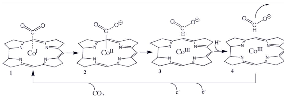
**Figure 4.** Target reaction between cob(I)alamin and  $\text{CO}_2$ , in the active site of EutB
