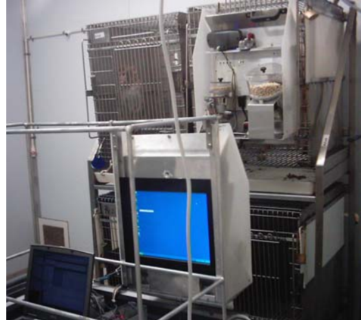
Figure 1. Two of the portable rigs used to test the monkeys. Front center: the touchscreen side of a rig. Rear left: a monkey in his home cage. Rear right: the back of a rig as it hangs on the cage.
