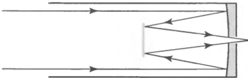
**Figure 11: Ray Diagram of Cassegrain Type Telescope<sup>2</sup>**
