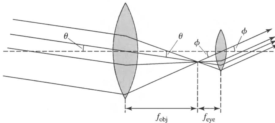
**Figure 12: Ray Diagram of Refractor Type Telescope<sup>2</sup>**
